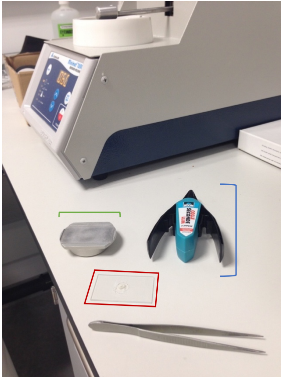
Figure 13. Photograph showing the sanding machine in the background, with the metal mount for the slide to be used in the sanding machine, to the left and marked in green. The ethyl cyanoacrylate used for mounting the samples to the slide to the right and marked
